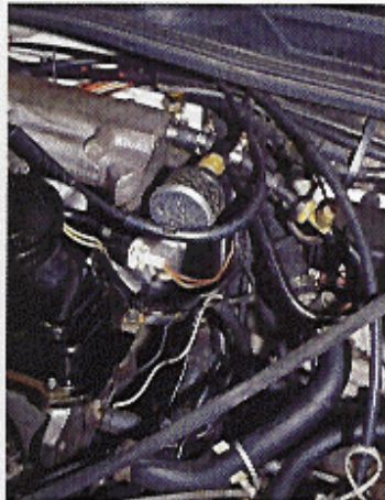
The unit is installed in-line with the manifold feed to the servo using jubilee clips. No hoses need to be cut.
